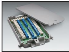
The Model 7708 plug-in module offers 40 channels of 2-pole or 20 channels of 4-pole multiplexer switching that can be configured as two independent banks of multiplexers. The built-in CJC sensors automatically linearize thermocouples, making the Model 7708 ideal for RTD, thermistor, and thermocouple temperature applications. It is also well suited for mixedsignal measurement applications that require multi-point monitoring, such as environmental stress screening.
